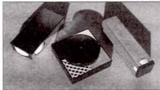
Figure 10: Conceptual side-selection prototypes. The force-feedback wheels mode is chosen by pressing the wheel at a specific position (left and right prototypes) or a position on the wheel's base (center). Since activation location is grounded relative to hand position, the selector is easy to find.
