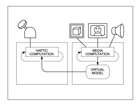
Peripheral model for haptic device Like mouse or keyboard Application dominant interface Haptic device is seen as "display"
