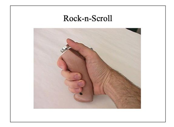
Game-like interaction – one hand Actuated wheel, with passive sprung 2<sup>nd</sup> axis Hand size, ergonomics
