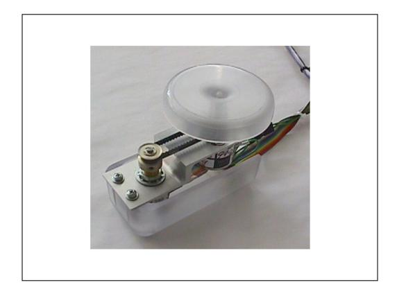
Brake – Passive haptic display
