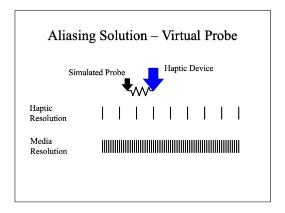
Virtual Probe – solution to aliasing
