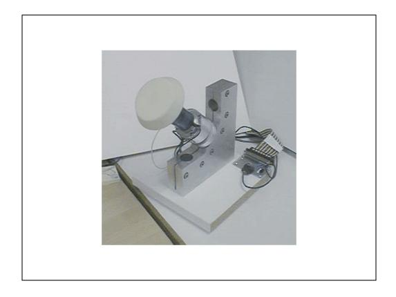
Orthogonal force SENSING – actuate in 1 DOF, but sense in > 1 – can be used, for example, to give users illusion of selectively engaging with the system
