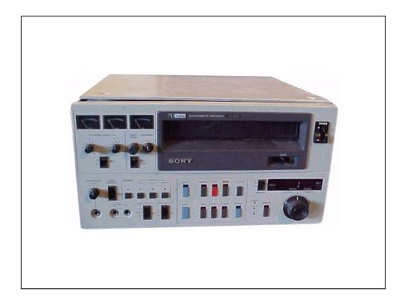
Means for finding footage with videotape -jog/shuttle wheel
